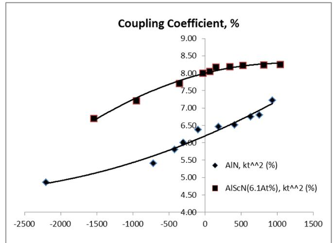
Tight control of coupling coefficient is essential for producing high quality devices. Using dual target magnetron configuration allows very tight control of stress and coupling coefficient across a wafer.
