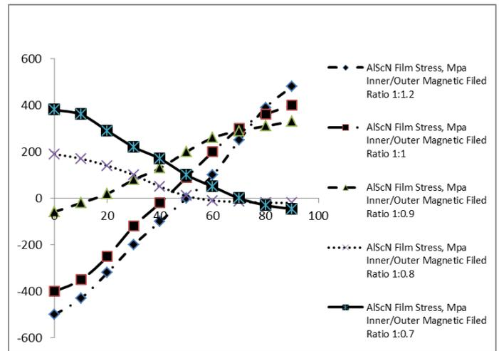
It is clear that a standard 1:1 ratio of magnetic field that produces the best results for AlN process is unacceptable for AlScN process. We found that the ratio of inner/outer of 1.0/0.8 is the best for stress control.
